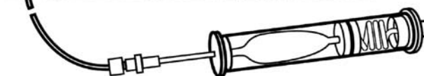
FIGURE 1. (A) The infusor consists of pressure applied by an elastomeric reservoir flowing through a restrictor that controls the rate of infusion. (B) The catheter is placed in the patella tendon defect.
